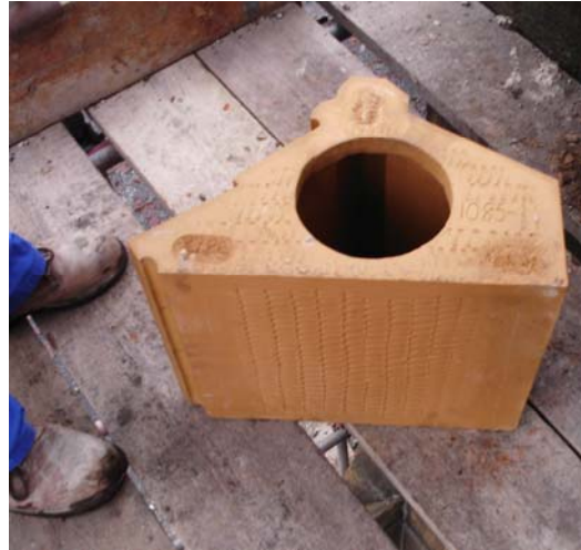
Fig. 5.24 Detail of new hollow terracotta block
